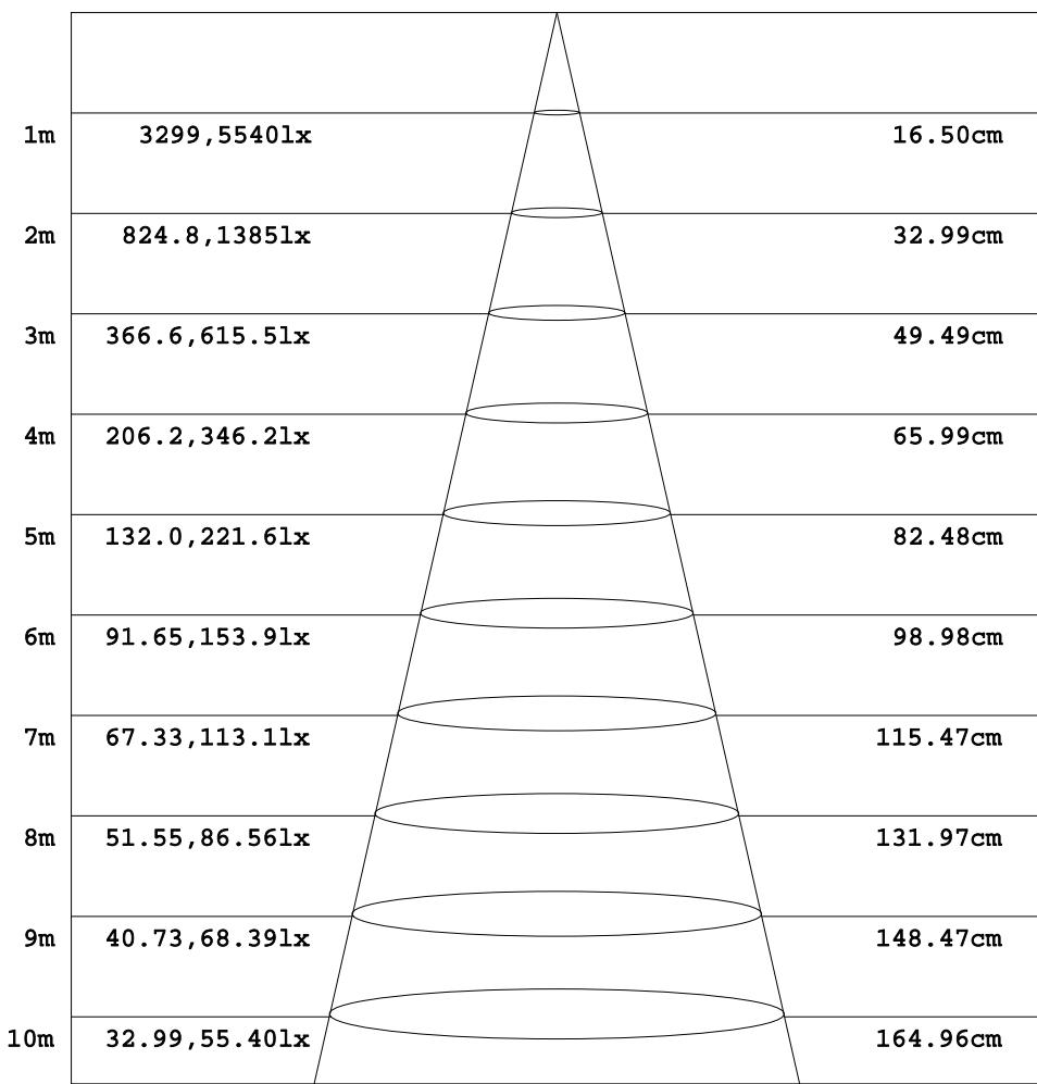
Height      Eavg , Emax      Angle:9.43deg      Diameter
