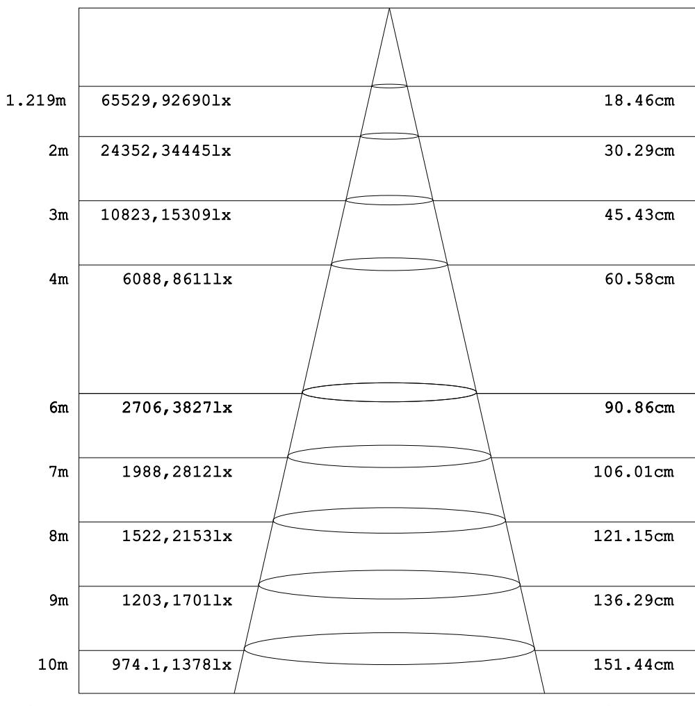
Height      Eavg, Emax      Angle: 8.66deg      Diameter
